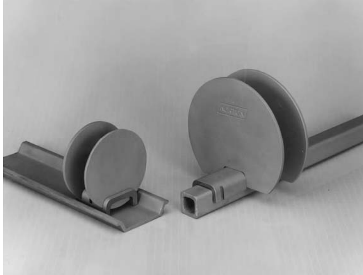
Figure 7.10. Supports for diffusion ovens of the semi-conductor industry (courtesy of St Gobain-Norton)
